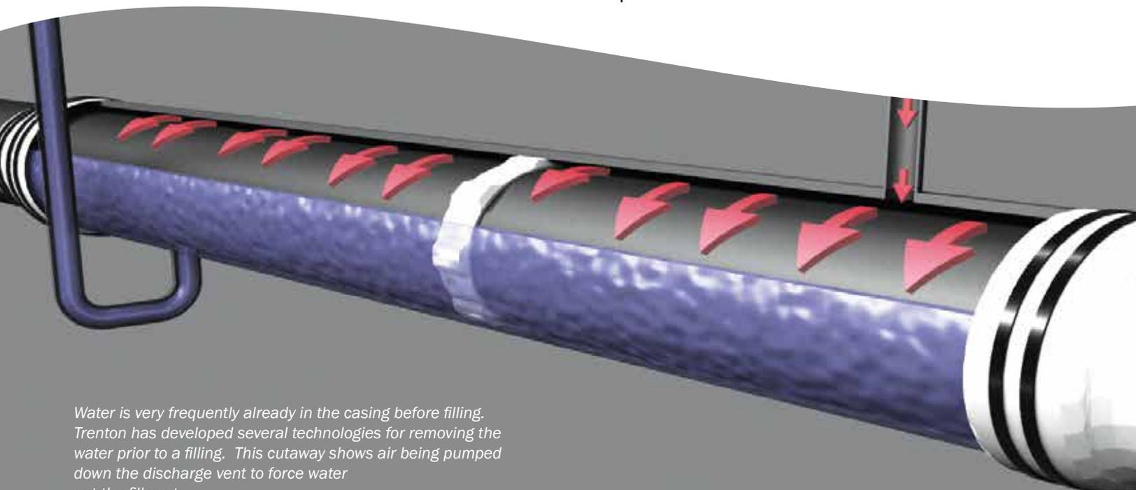
*Water is very frequently already in the casing before filling. Trenton has developed several technologies for removing the water prior to a filling. This cutaway shows air being pumped down the discharge vent to force water out the fill vent.*
